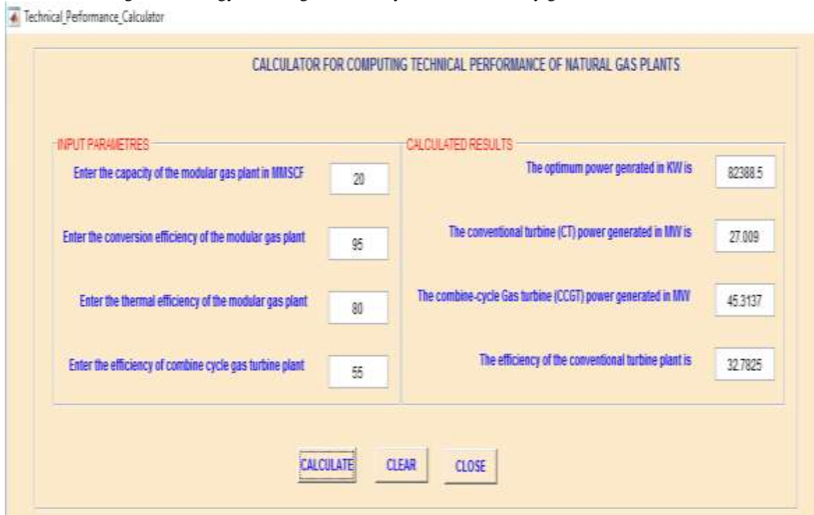
Figure 5: MATLAB Calculator Program for Calculation of Technical Performance Parameters
